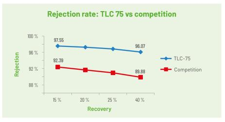
Testing conditions: 75 gallon per day RO membranes, 3.5 bar feed pressure, 1000 ppm of TDS, softened water.
